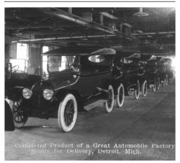
Row of completed Model T's come off the Ford assembly line, about 1917.<sup>15</sup>
